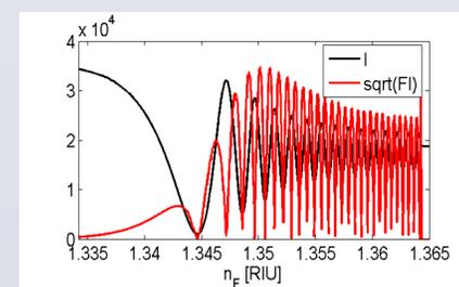
Figure 5: Interferometer output and the Fisher information calculated for the porous-film MZI.
