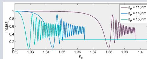
Figure 3: a) Schematic of a MZI. b) Intensity output of the MZI with a fixed porosity  $P = 32\%$  and  $d_p$  as a design parameter.
