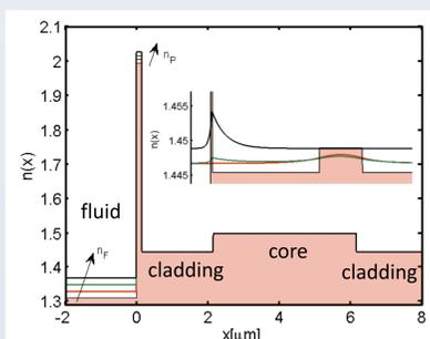
Figure.1 Refractive index profile of the sensor together with influence of fluid refractive index on the mode profile.
