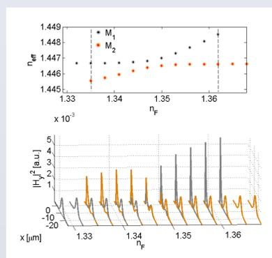
Figure.2 (a) Mode effective indices as functions of the fluid refractive index. (b) The corresponding mode field intensities. The film thickness was  $d_p=140\text{nm}$  and porosity  $P=32\%$ .
